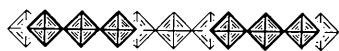
Fig. 3. Characteristic feature of Nb_2O_5 , three octahedra (heavier outline) sharing edges with three at a level y=\frac{1}{2} above and below (lighter outline); an S unit, found in related phases (Wadsley, 1961; Andersson, 1963).
